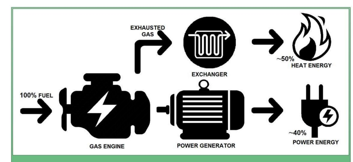
Cogeneration technology is the combined generation of electricity and heat energy. Cogeneration technology allows to use the heat of exhaust gas takes off in special heat exchangers, thereby the overall coefficient of fuel utilization increases and harmful influence on the environment reduces
